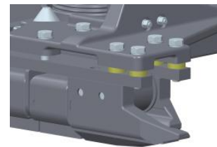
Magnet end piece with welded Friction elements
