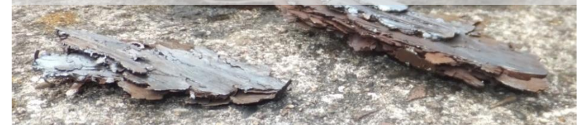
Severe „weldings“ on steel pole shoes
