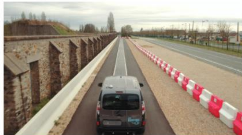
A Renault Kangoo BEV is charged while driving the FABRIC test track in Versailles, France.
